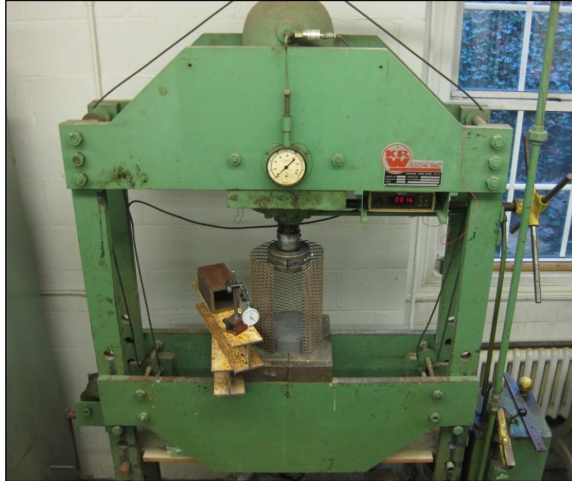
Figure 7. Hydraulic universal testing machine. A digital read out was used to display loading of the samples and a dial gauge was used record axial deflection of the sample.
