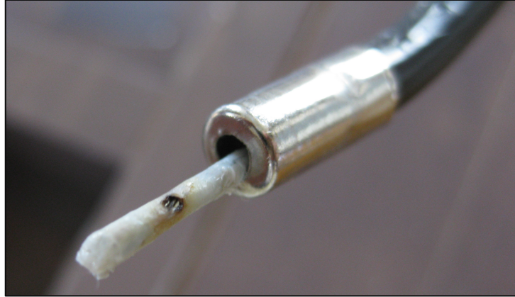
Figure 15. The damaged first shutter.
