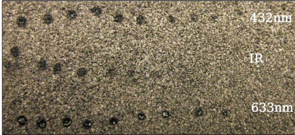
Figure 3. The results of the wavelength sensitivity tests. Dwell time decreases from left to right from 10 seconds to 1 second.
